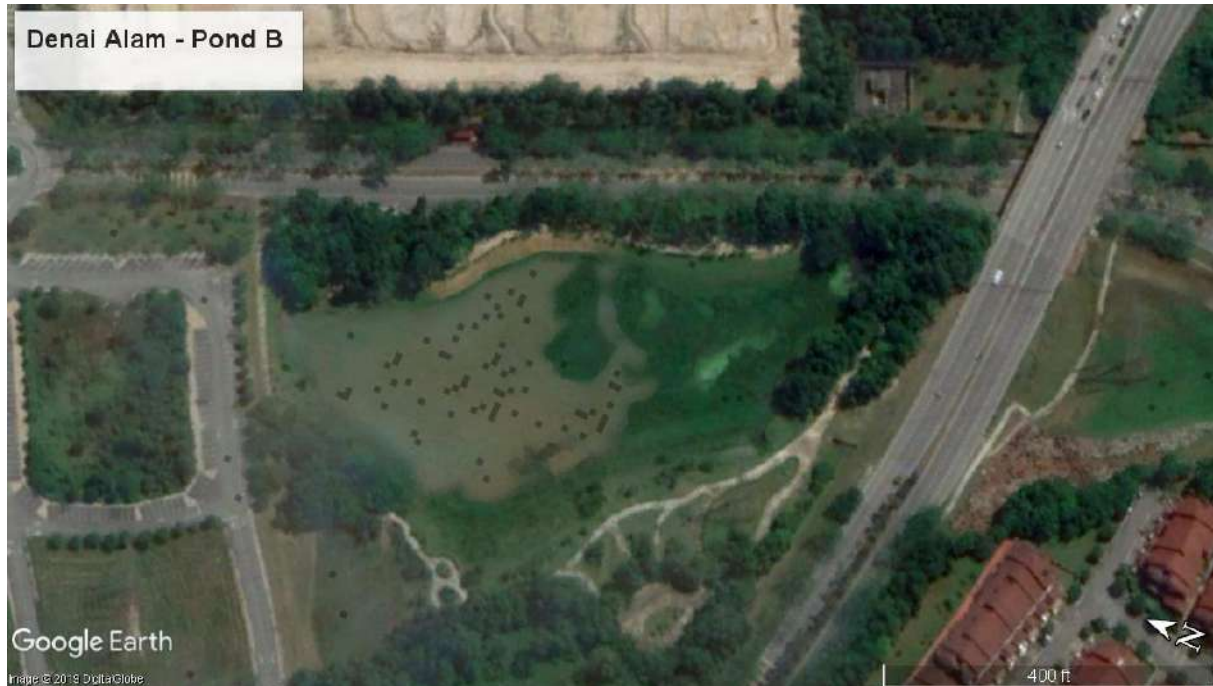
Figure 3: Google Earth satellite image (6-12-2017) of Denai Alam Pond B showing extent of maturity of the pond, and evidence of its eutrophic status in the South-East section of the pond.
