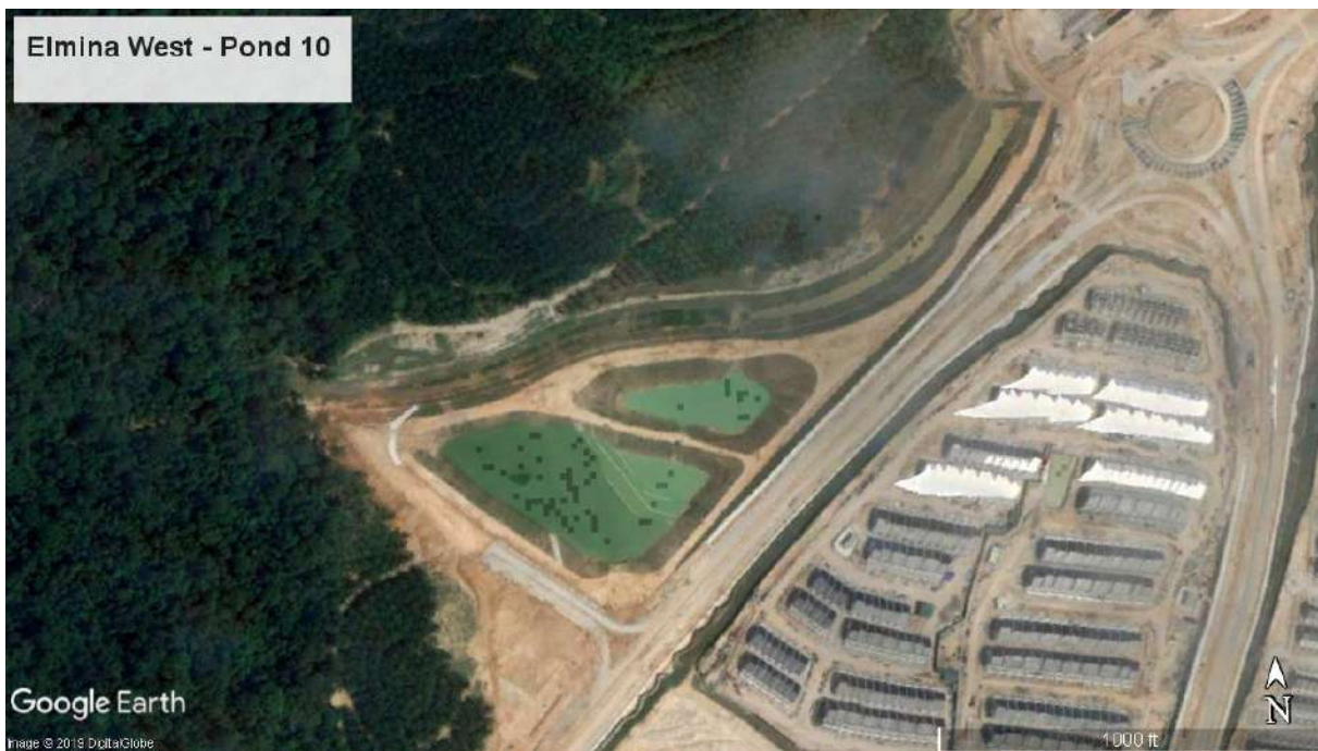
Figure 23: Google Earth satellite image (6-12-2017) of Elmina West Pond 10 showing proximity to edge of Bukit Cherakah Forest Reserve (on the left), terracing of upper pond and in-flow sluices to the Sungai Subang to the north-east.
